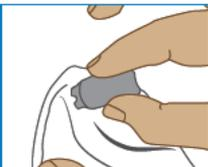
Clean the back of your transmitter with an alcohol wipe.
