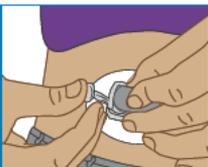
Place one finger on the transmitter to keep it in place. With your other hand, pull the transmitter latch up and forward until you hear 2 clicks.
