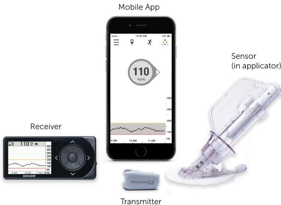
The sensor (Figure 12) is minimally invasive and measures glucose concentrations in the interstitial fluid. The sterile sensor is inserted into the subcutaneous tissue of the abdomen for adult patients and abdomen or upper buttocks for pediatrics. The sensor can be worn for up to seven days and is adhered to the skin with an adhesive patch.
