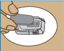
Place the transmitter in the sensor pod with the flat side down, and thinner side away from the transmitter latch.
