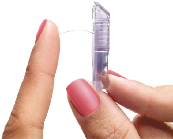
The transmitter (Figure 13) is lightweight, reusable for up to three months, and water resistant, allowing for use during bathing or swimming. The transmitter samples the electrical current produced by the sensor and converts these readings into glucose values using an onboard algorithm.
