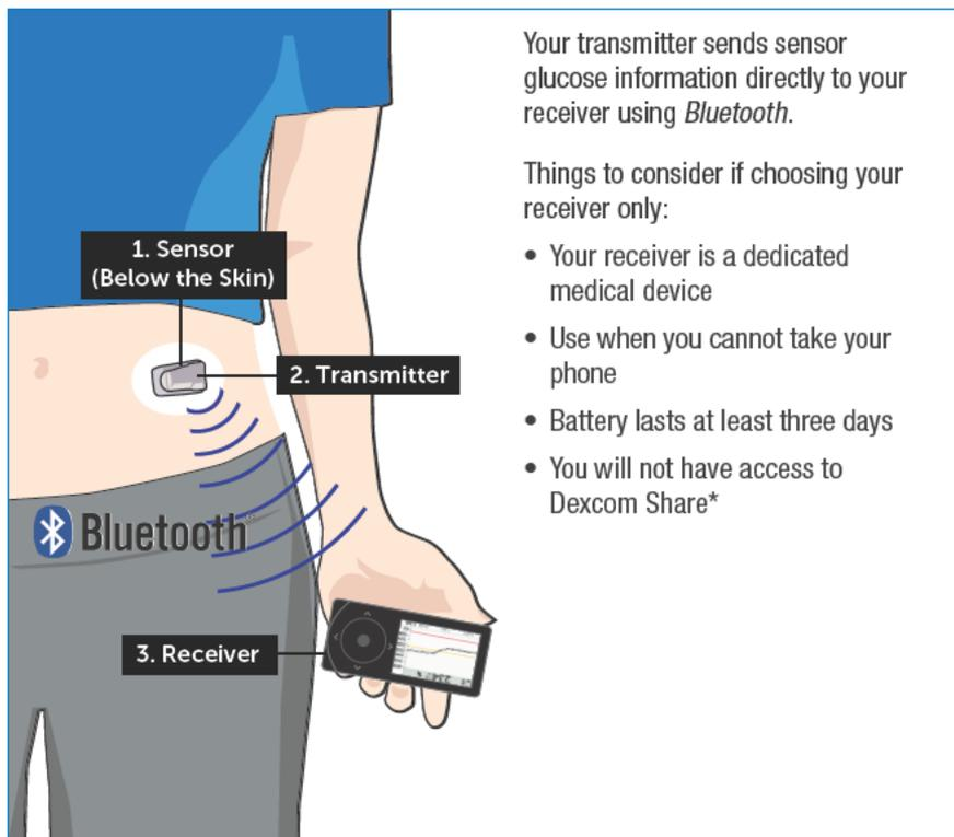
Your transmitter sends sensor glucose information directly to your receiver using *Bluetooth*.
