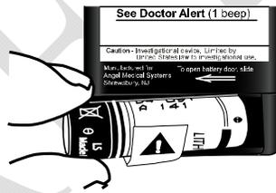
4. Close the battery compartment by sliding the battery cover completely to the right.
