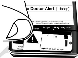
3. Insert the positive (+) end of the new battery into the battery compartment, and then push down on the battery's negative (-) end. Be sure that the tab is exposed for subsequent removal.
