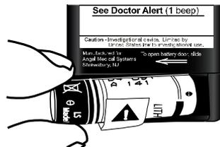
4. Close the battery compartment by sliding the battery cover completely to the right.
