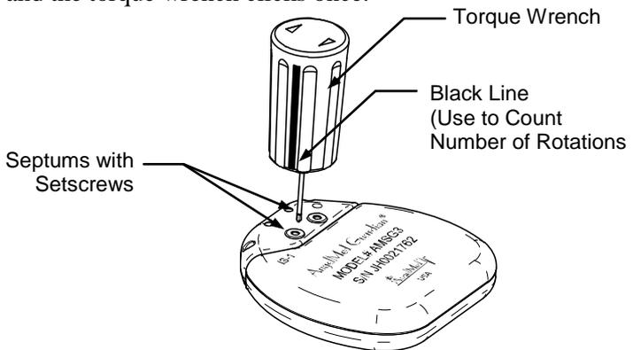
2. Observing the black line on the torque wrench handle, turn the same setscrew counterclockwise six full rotations to provide clearance for the lead connector pin.
