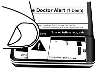
3. Insert the positive (+) end of the new battery into the battery compartment, then push down on the battery's negative (-) end.
