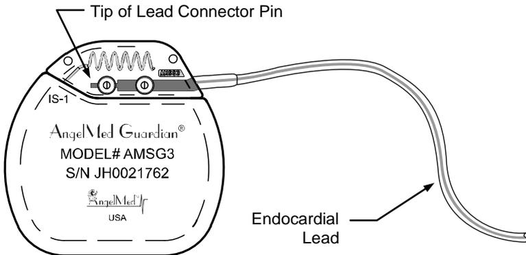
6. Insert the torque wrench through either IMD header septum and into a setscrew. Turn the setscrew clockwise until the torque wrench clicks once.
