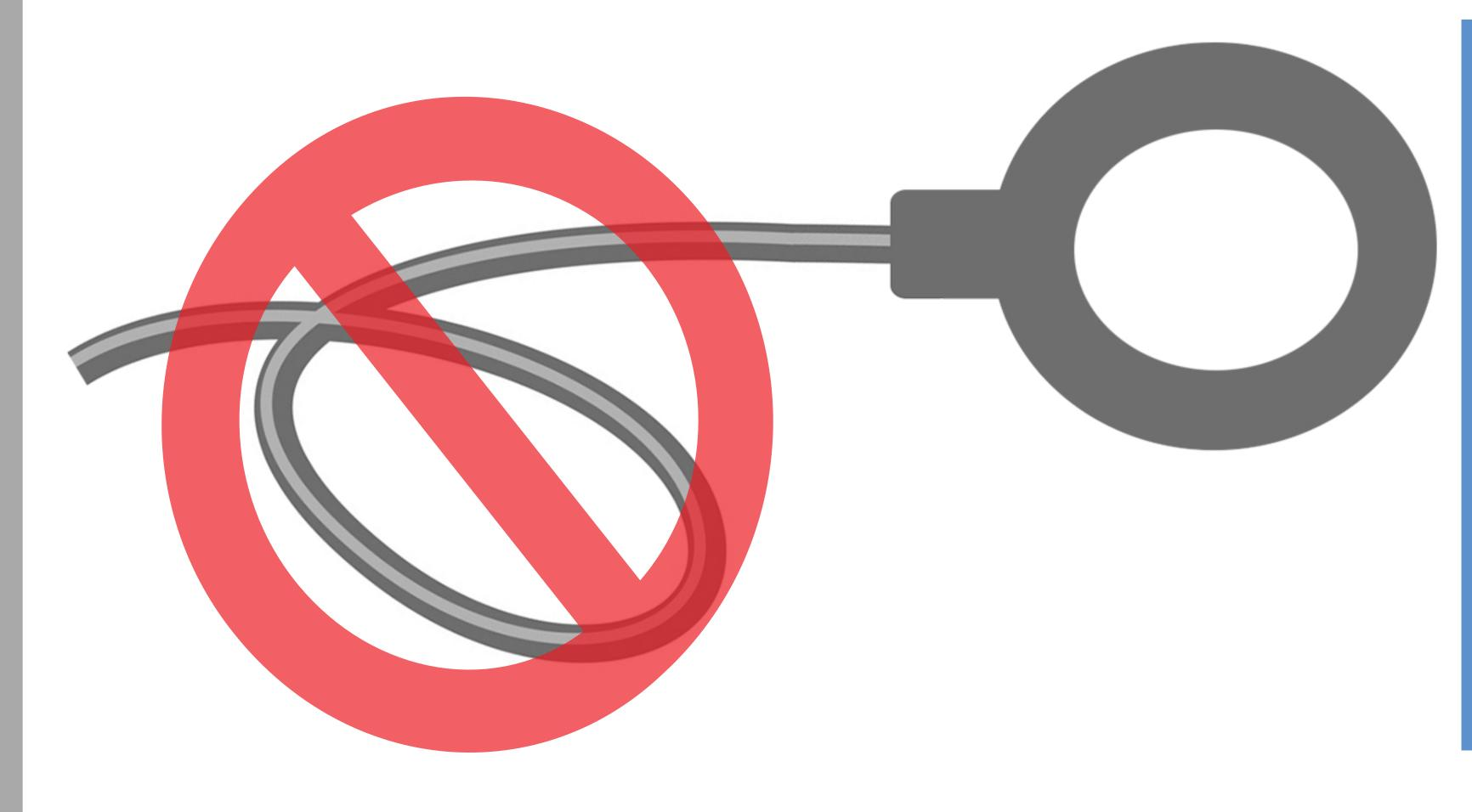
Route cables out of the scanner in a straight line. Don't coil cables or allow them to touch the patient.
