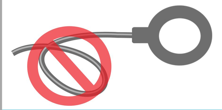
Route cables out of the scanner in a straight line. Don't coil cables or allow them to touch the patient.
