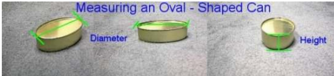
Figure 14 – Measurement of an Oval Shape Container
