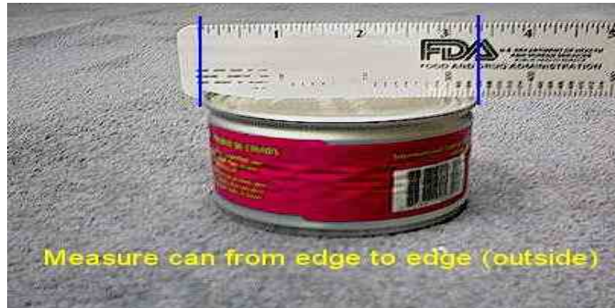
Figure 15 – Measurement of Outer Edges of Container
