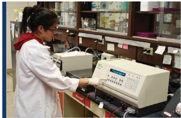
Microbiologist Julie Bentzoni performing DNA fingerprinting using PFGE (pulse field gel electrophoresis). This PFGE tool separates DNA molecules by applying an electrical field to a gel matrix.
