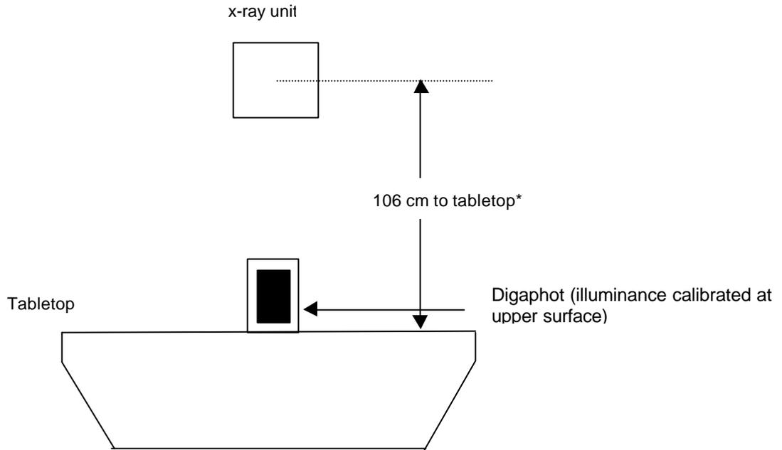
Figure 2 Digaphot positioned for measurements in the upright position
