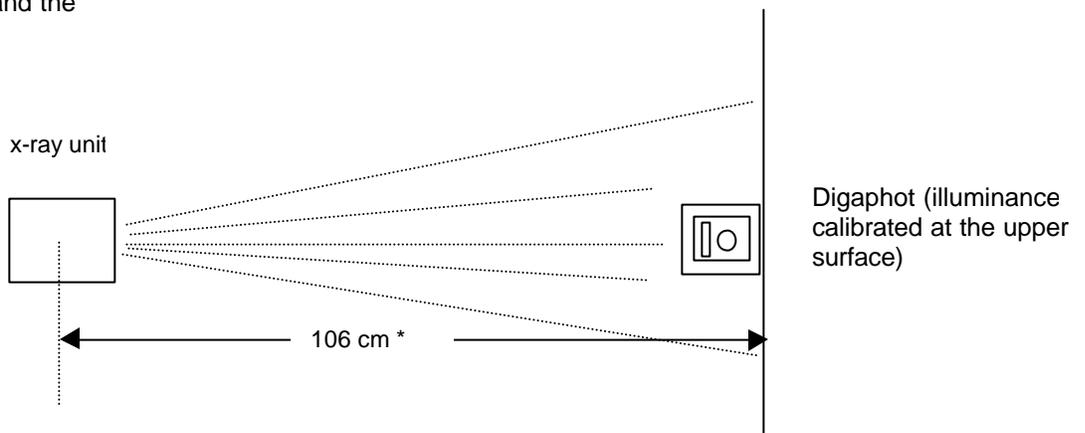
Figure 3 Digaphot Positioned for Measurement in the Horizontal Position
