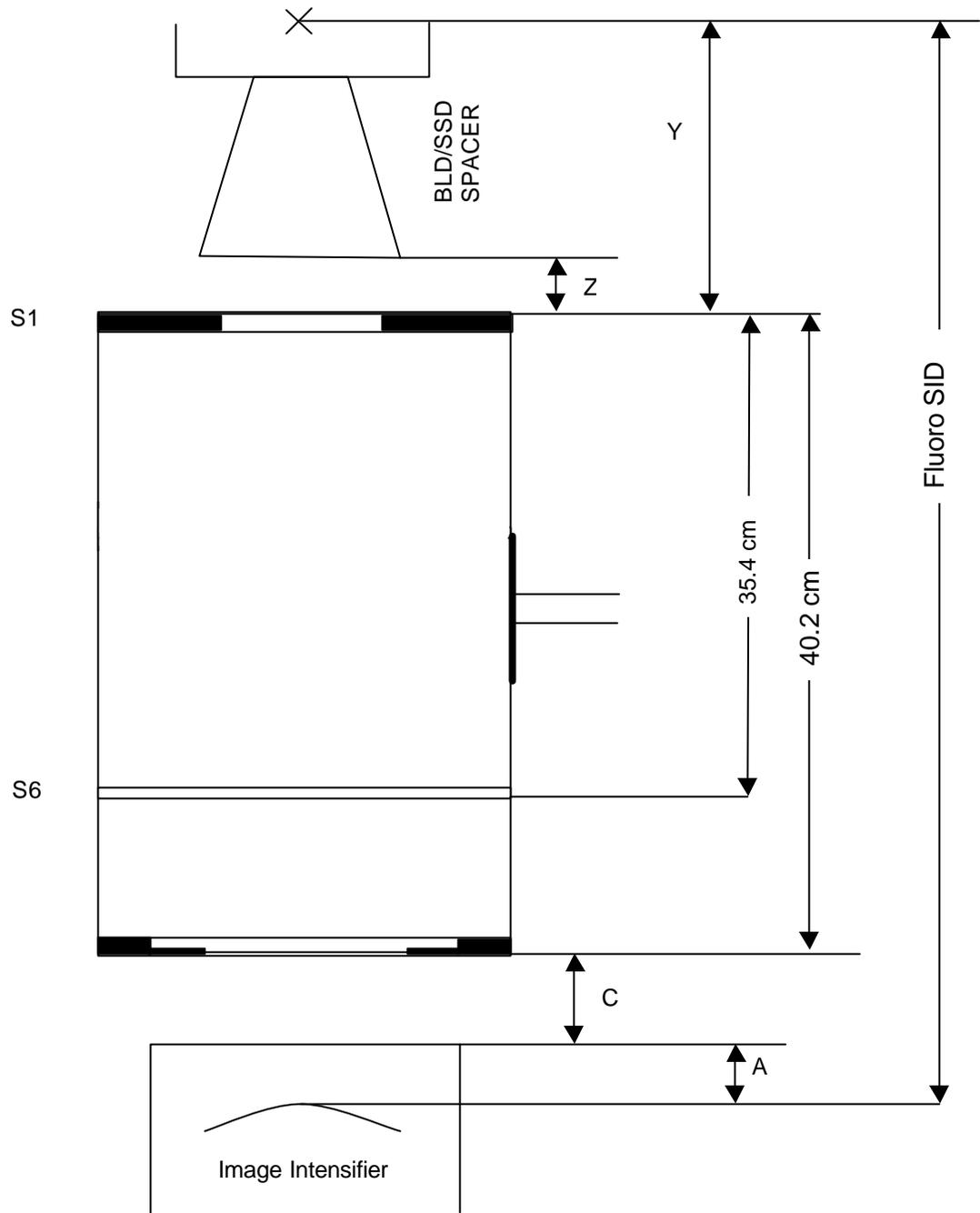
A = Distance from input phosphor of the image intensifier to the face of the image intensifier (supplied by manufacturer, if not available use 3.0 cm which is a representative value)
