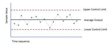
When a process is stable and in control, as in the above example, you see nothing but *common cause variation*. This results from the normal operation of a system and is expected due to routine factors.
