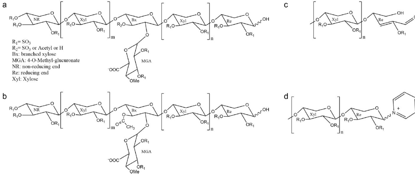
**Fig. 1** The chemical structure of pentosan polysulfate sodium (PPS) backbone (a) and its modifications of acetylation (b) in branched xylose, aldehyde (c) and pyridine (d) addition at the reducing ends. Integer numbers m and n may take values from 0 to 26 (22)
