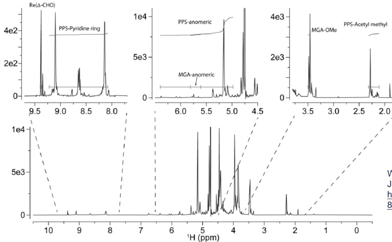
Fig. 2 The representative PPS 1D  $^1\text{H}$  qNMR spectrum with integration ranges shown in the three sub-spectra
