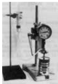
Figure 24. Can piercer and gas collection apparatus.
