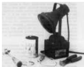
Figure 7. Ultraviolet light for fluorescein dye test.
