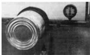
Figure 8. Application of vacuum for fluorescein dye test.
