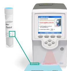
**6** Turn the assay tube. Remove the assay tube sleeve and then insert the assay tube into the analyzer tube entry door. Processing begins automatically.
