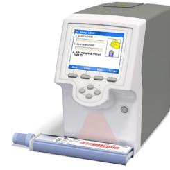
**6** Turn the assay tube. Remove the assay tube sleeve and then insert the assay tube into the analyzer tube entry door. Processing begins automatically.
