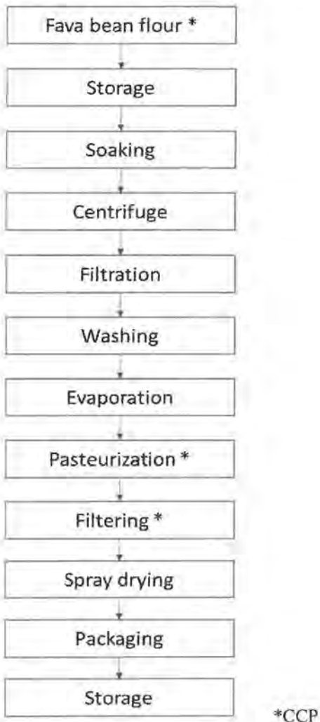
Figure 1. Steps in the fava bean protein production process
