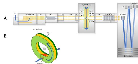
Figure 1. Instrument diagrams of (A) cyclic IM (cIM)-MS used in this study and (B) cIM device. Adapted from [1].
