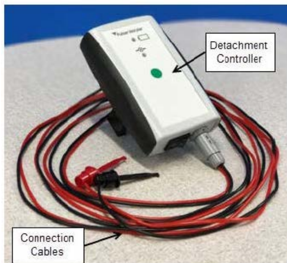
Figure 4: PulseRider Detachment System
