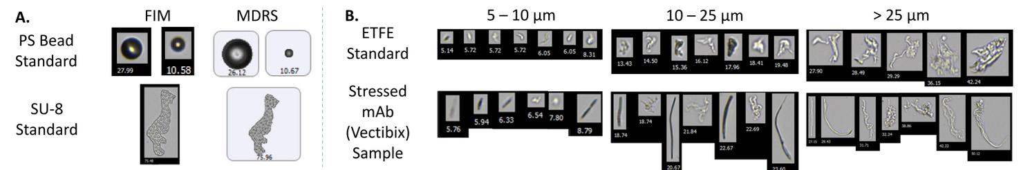
**Figure 1.** Representative images of polystyrene (PS) bead standard, SU-8 standard, ETFE standard, and particles found in a stressed mAb sample. (A) Images of monodisperse particles (PS beads on top and SU-8 on bottom) captured by FIM (left) and MDRS (right). (B) Images of polydisperse particles (ETFE on top and mAb on bottom) captured by FIM. Vectibix was subject to a combined stress (70 C and 300 rpm) for 30min.
