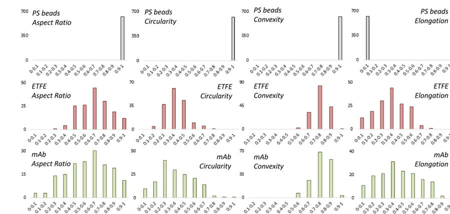
**Figure 3.** Morphological data histograms of polystyrene beads, ETFE standard, and a stressed mAb (Vectibix) stressed measured by MDRS.
