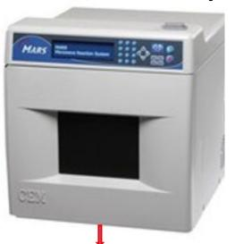
0.5g of sample + 8 mL HNO<sub>3</sub>, 1mL H<sub>2</sub>O<sub>2</sub> + 1mL HCl Step 1: 1600W 20 min to 120°C for 5 min Step 2: 1600W 20 min to 200°C for 25 min
