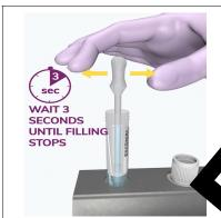
12b. ...let go of pipette completely and allow to fill.
