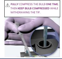
15. To dispense sample:Squeeze bulb only ONCE, and compress fully.
