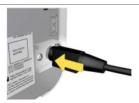
2. Connect adapter to rear power port with flat side facing left as shown.
