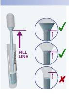
Open sample port and insert pipette tip. Squeeze firmly ONCE; while holding, remove from Cartridge.
