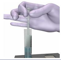
**12**a. Still squeezing the bulb, submerge tip in tube liquid, **then...**
