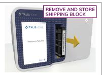
**5.** After Welcome screen appears, remove ejected shipping block and set aside.
