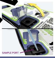
**14.** Open sample port lid and insert pipette tip into the port.
