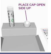
Uncap control prep tube and place in cartridge preparation tray.
