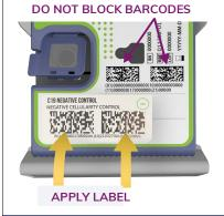
**8.** Remove Cartridge from pouch, place in tray and apply C19 Control Label (from Step 1b).
