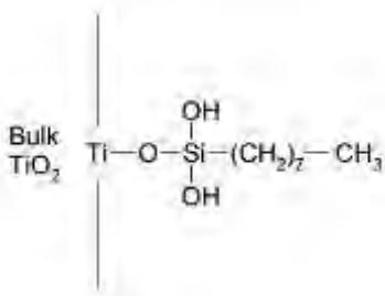
In the manufacturing process, titanium dioxide, OTES and other raw materials were reacted under certain temperature. After the reaction, Octyltriethoxysilane (OTES)-modified titanium dioxide (FCS) was obtained. The FCS has high dispersibility and melt flow with excellent whiteness and blue undertone. The silane modification aims to create a surface that is more compatible with the resin system and enables the FCS to disperse better in resins.
