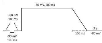
Data derived from this protocol are used to understand the relationship between drug potency on affecting hERG current and therapeutic exposure level. Seal resistance should be  $\geq 1G\Omega$ . This voltage protocol is to be repeated every 5 s. The voltage "ramp down" phase is 100 ms in duration, from +40 mV to -80 mV
