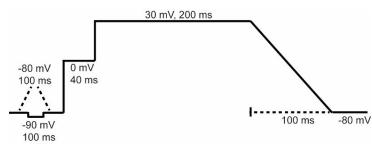
$Ca_V 1.2$  current amplitude (leak current-subtracted or verapamil subtracted and not raw value) is measured at two places – as the peak inward current at the 0 mV step and as the peak inward current evoked at the "ramp down" phase (+30 to -80 mV ramp down in 100 ms). If possible, at the end of the
