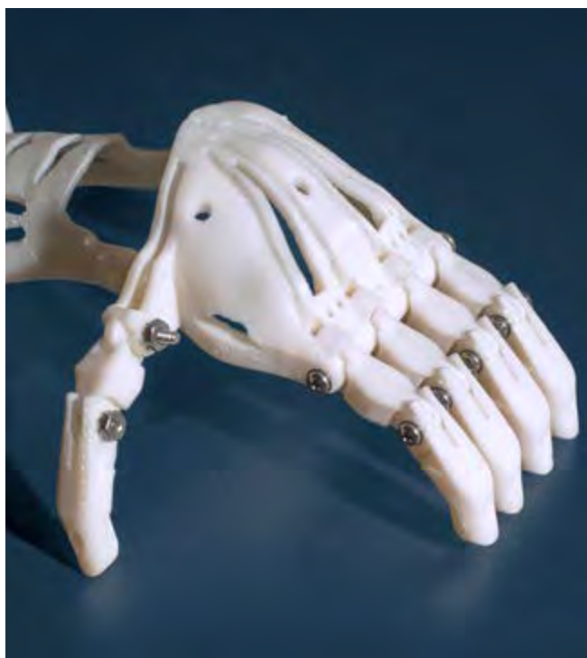
This 3-D printed prosthetic hand was printed and assembled by FDA researchers in their CDRH laboratory.
