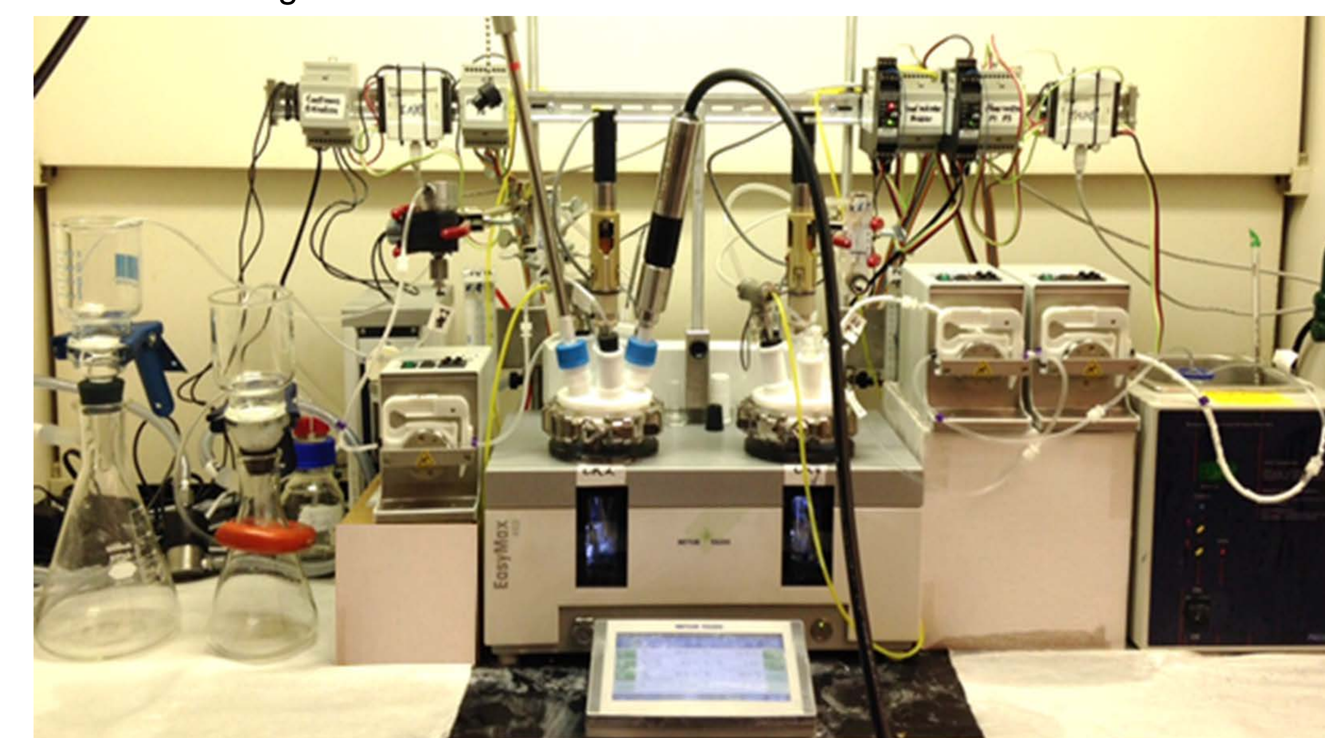
Figure 4. Two-stage MSMPR system with implemented PAT tools and periodic filtration unit.
