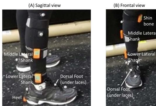
Figure 1: IMU placements on the lower leg.
