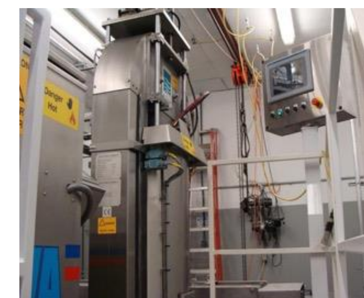
Figure 1. Avure 24L unit within IFSH pilot plant.
