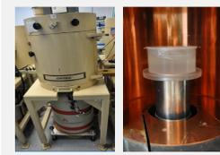
Figure 1. High purity germanium detector (HPGe) (Left) Inside gamma detector shielding (Right)
