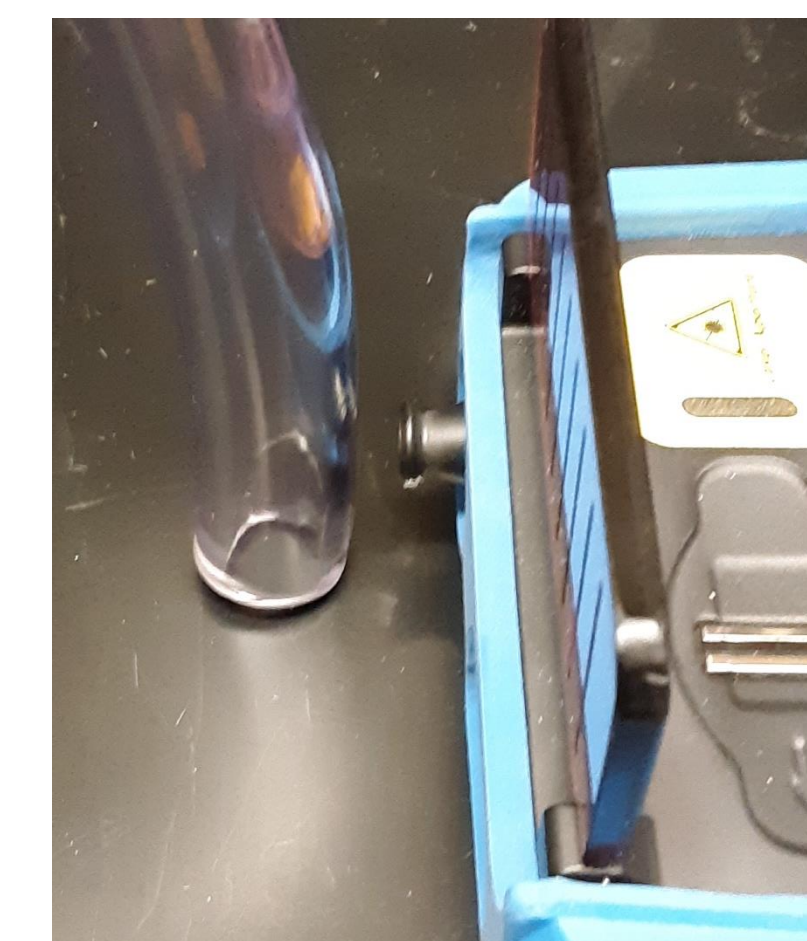
785nm Raman instrument with fixed probe cone
