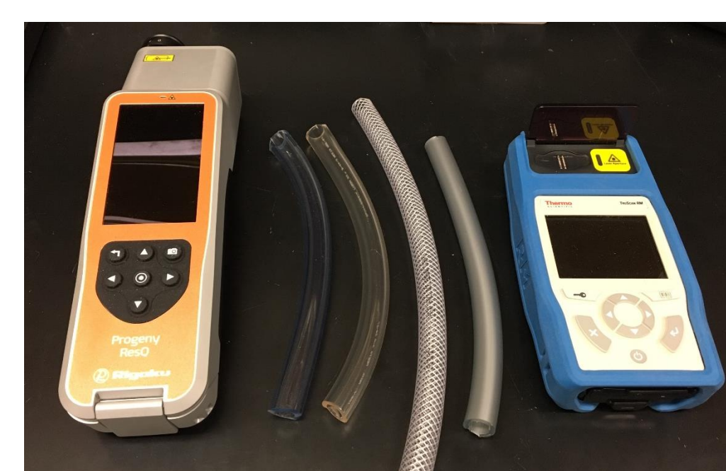
Figure 1: 1064nm (Left) and 785nm (Right) portable Raman instruments, with food contact production line tubing (Middle).
