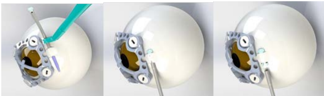
Figure 6 Placement of VisAbility Micro Inserts with VisAbility Feeder Tube
