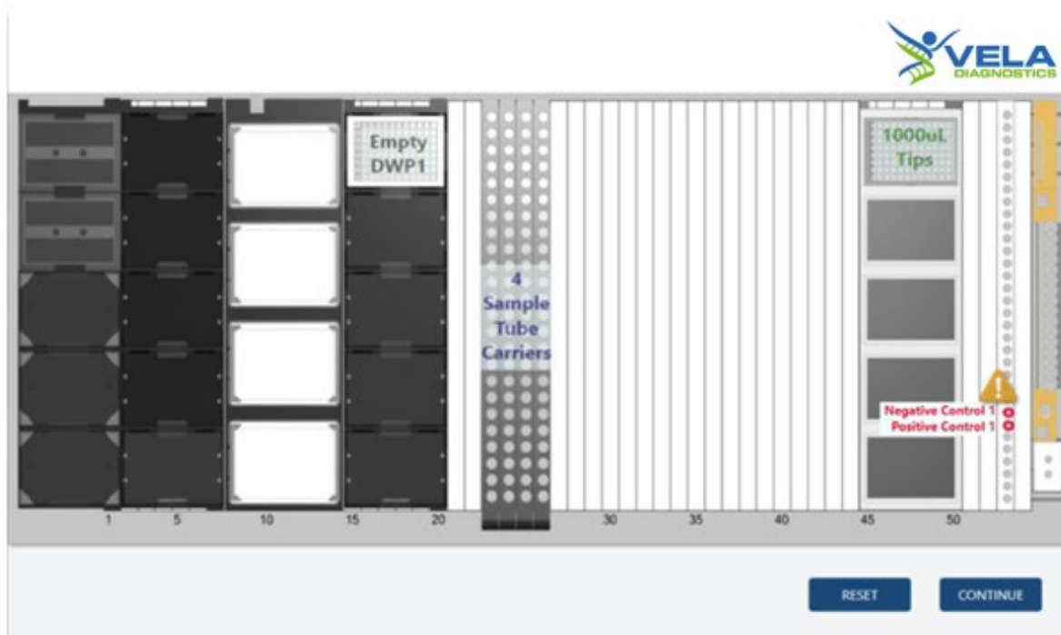
Figure 4. Layout of the Hamilton Microlab STAR platform for 1 deepwell plate (1x96 tests) for sample plate preparation (refer to Appendix for 2 to 4 deepwell plates layout).
