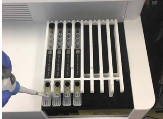
*Figure 4: Adding Controls to the Cartridge*
