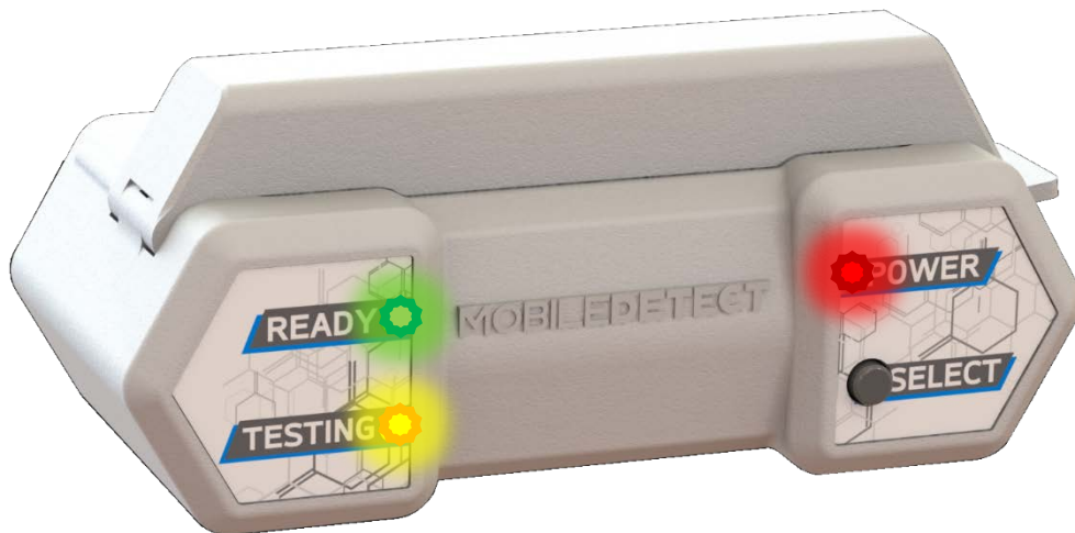
Figure 2: MD-Bio BCC19 Heater when in Error Mode
