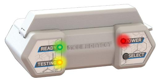
Figure 2: MD-Bio BCC19 Heater when in Error Mode
