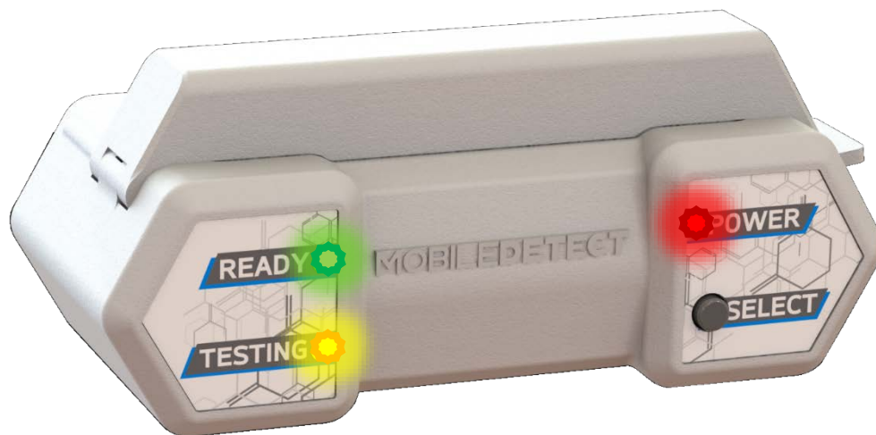
Figure 2: MD-Bio BCC19 Heater when in Error Mode
