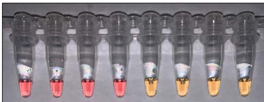
Figure 8: Example of Test Results (4 Left Negative, 4 Right Positive)
