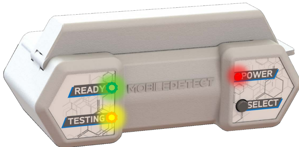
Figure 6: MD-Bio BCC19 Heater when Test is Completed
