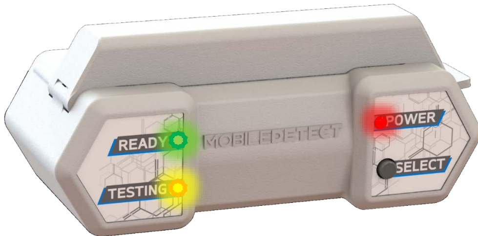
Figure 6: MD-Bio BCC19 Heater when Test is Completed
