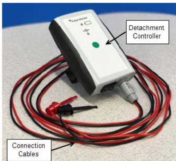
Figure 4: PulseRider Detachment System
