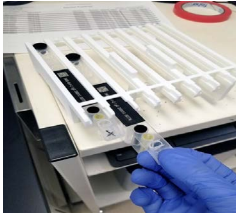
Figure 3: Inserting Controls Cartridges into Reagent Rack
