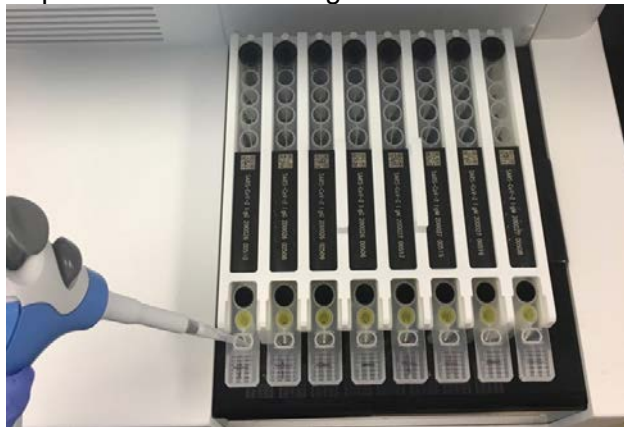
Figure 4: Adding Controls to the Cartridge
