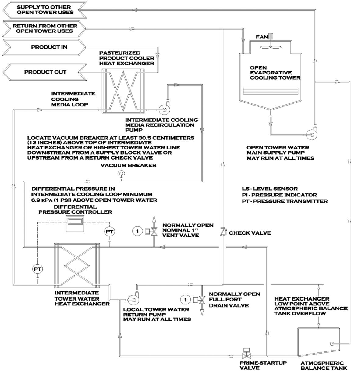
① THIS VALVE MUST AUTOMATICALLY OPEN AND REMAIN OPEN WHENEVER THE REQUIRED PRESSURE DIFFERENTIAL IN THE INTERMEDIATE TOWER WATER HEAT EXCHANGER DOES NOT EXIST.
