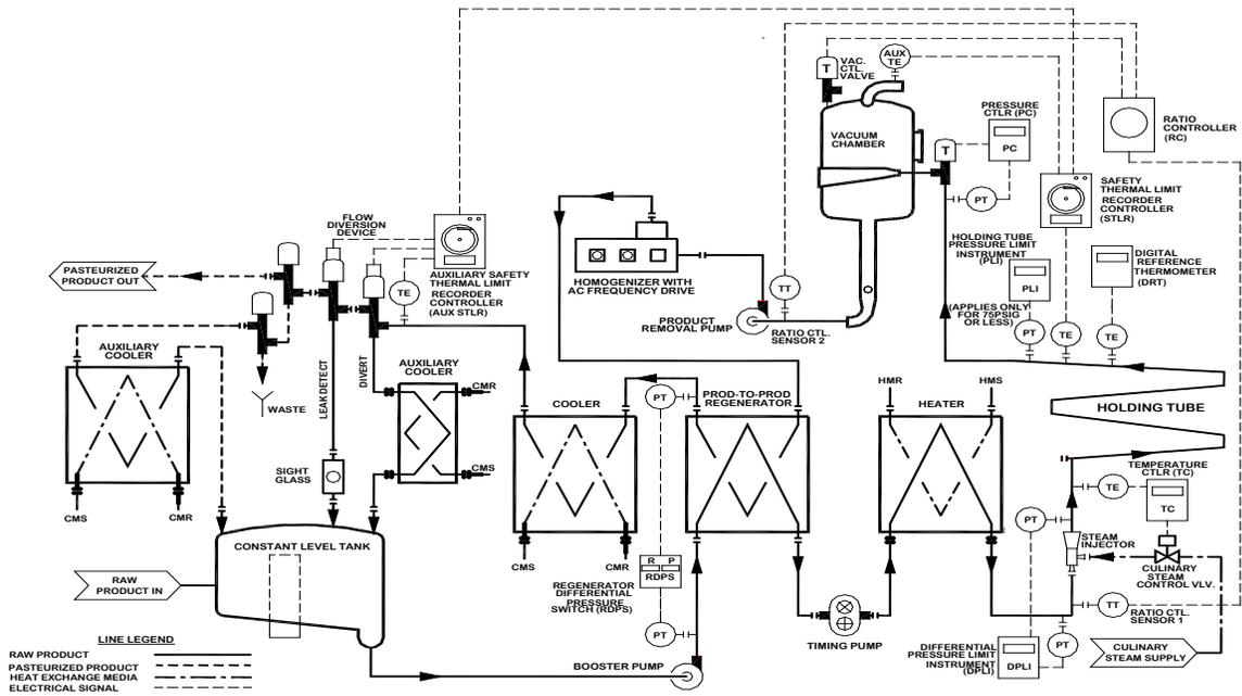
**Figure 41. HHST Pasteurizer Utilizing Steam Injection Heating, Vacuum Flash Cooling and a Flow-Diversion Device Located Downstream of the Cooler Section Pump**
