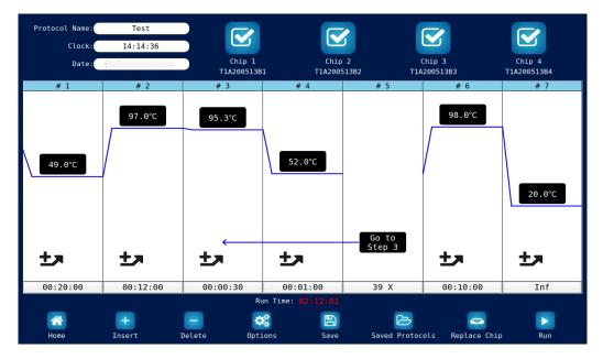
Figure 7. User interface for setting RT-Digital PCR thermal cycling protocol
