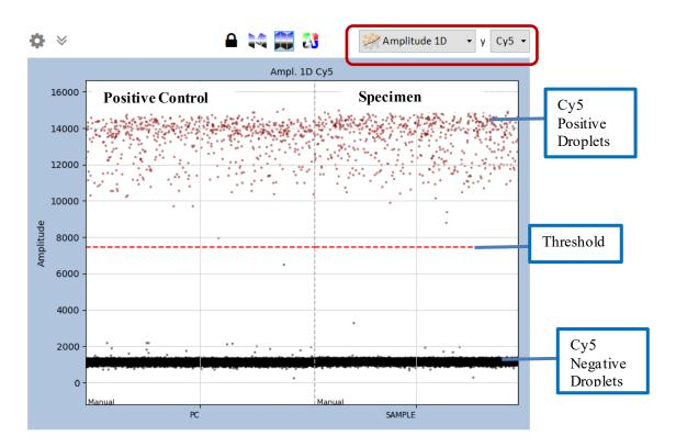
Figure 18. Thresholding specimens in Cy5 channel
