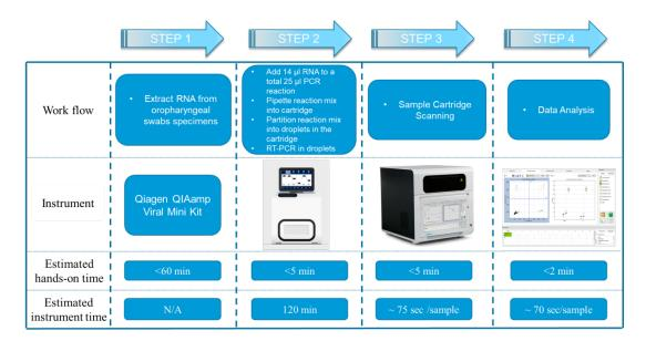
Figure 2. FastPlex Triplex SARS-CoV-2 Detection Kit-Digital PCR Workflow
