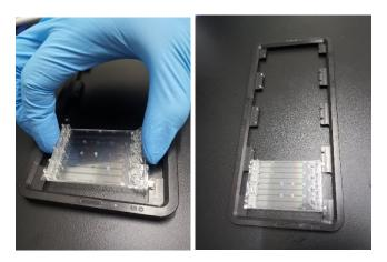
Figure 4. Place microfluidic cartridge on cartridge holder
