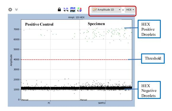
Figure 17. Thresholding specimens in HEX channel
