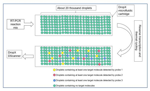
Figure 1. Principle of RT-Digital PCR
