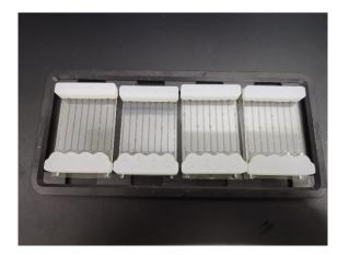
Figure 6. Microfluidic Cartridges in the holder
