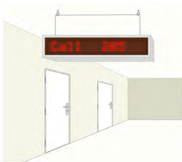
Figure 285. Ceiling mounted corridor display
