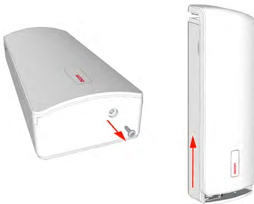
Figure 381. Removing the front cover of the NILF
