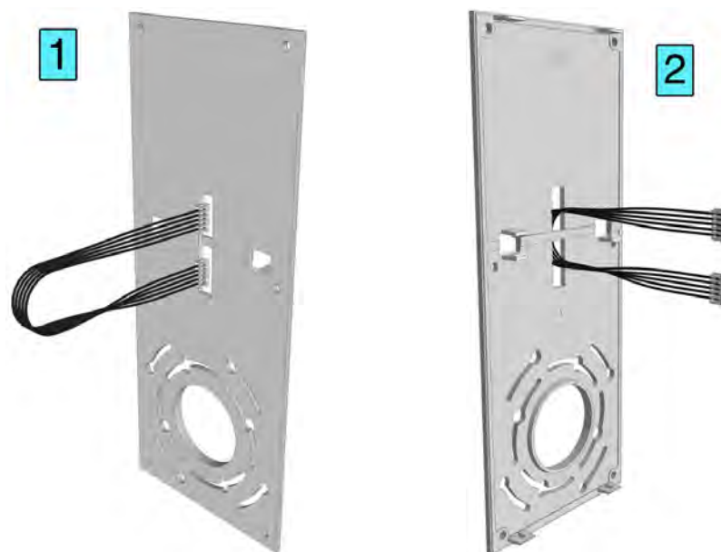
Figure 228. Inserting the connection cable through the backplate
