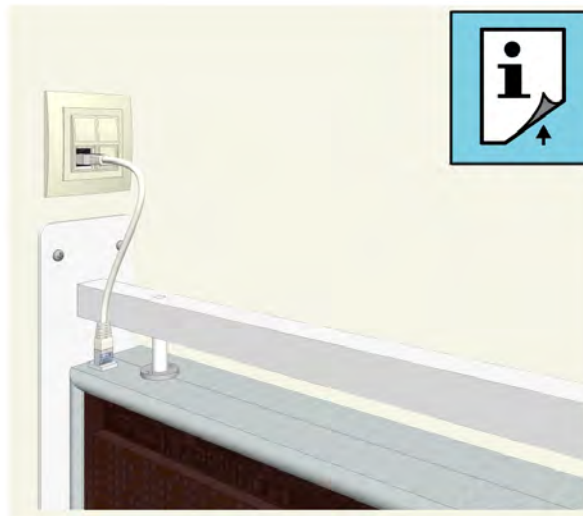
Figure 295. Connecting the displays ethernet cable
