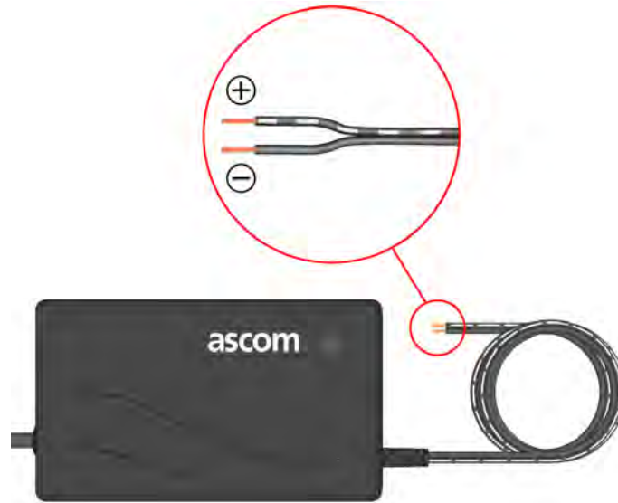
Figure 12. 24V/4.2A power supply unit output wires polarity
