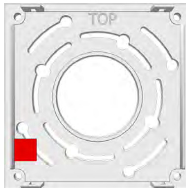
Figure 214. Placement of the adhesive tape onto backplate.
