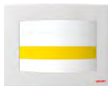
Figure 46. Fault indications on the NIRC3 yellow lamp
