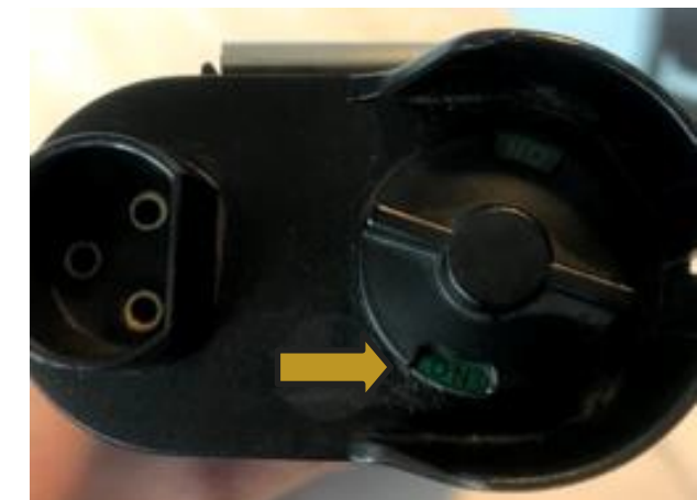
Battery in ON Position
