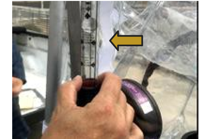
Attach Inner P100 Filters to PAPR Motor
