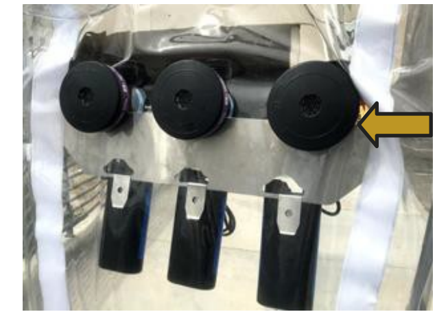
Attach Inner P100 Filters to PAPR Motor
