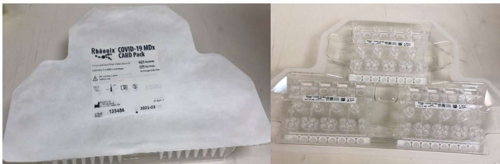
Figure 2. The Rheonix COVID-19 MDx Assay cartridge Pack. Left: Pack of three CARDS with pack cover in place. Right: Pack of three CARDS with pack cover removed.
