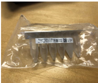
Figure 4. Rheonix COVID-19 MDx Assay PCR Mix, Pack B. Pack B ready for insertion into Pack A (Figure 3), at its designated location.
