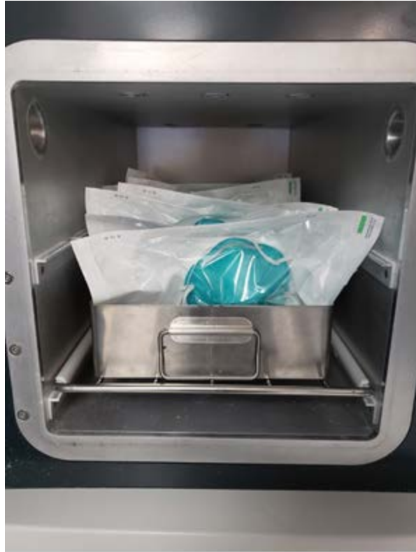
Figure 4: Sterilization basket with up to 12 individually packaged respirators, placed inside of the Sterilucient sterilizer.
