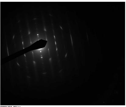
308004 FDA\_063.jpg Chrysotile 4 14:58 8/1/2019 TEM Mode: Diffraction Microscopist: ()) Camera: NANOSPRT5, Exposure: 800 (ms) x 5 drift frames, Gain: 1, Bin: 1 Gamma: 1.00, No Sharpening, Normal Contrast
