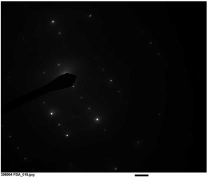
308004 FDA\_UTs.jpg Tremolite 16:36 7/29/2019 TEM Mode: Diffraction Microscopistic for Microscopistic for Camera: NANOSPRTS, Exposure: 800 (ms) x 5 drift frames, Gain: 1, Bin: 1 Gamma: 1.00, No Sharpening, Normal Contrast
