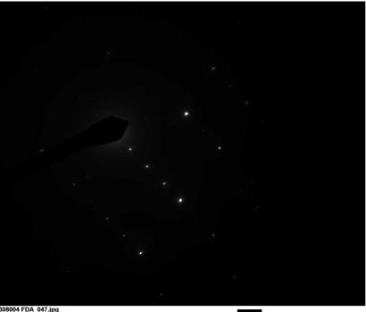
308004 FDA\_047.jpg Tremolite 1 18:14 7/30/2019 TEM Mode: Diffraction Microscopist. Camera: NANOSPRT5, Exposure: 800 (ms) x 5 drift frames, Gain: 1, Bin: 1 Gamma: 1.00, No Sharpening, Normal Contrast
