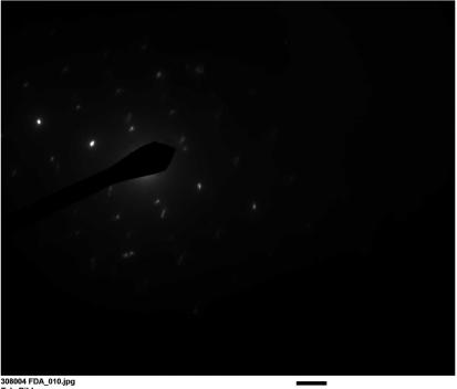
308004 FDA\_010.jpg Talc Ribbon 15:45 7/29/2019 TEM Mode: Diffraction Microscopist: Tem Tem Code: Diffraction Camera: NANOSPRT5, Exposure: 800 (ms) x 5 drift frames, Gain: 1, Bin: 1 Gamma: 1.00, No Sharpening, Normal Contrast
