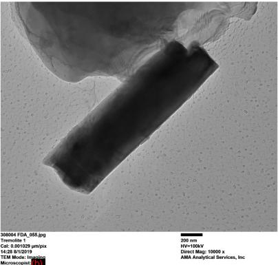
308004 FDA\_055.jpg Tremolite 1 Cal: 0.001029 µm/pix 14:28 8/1/2019 TEM Mode: Inaging Microscopist 1 Camera: NANOSPRT5, Exposure: 800 (ms) x 5 drift frames, Gain: 1, Bin: 1 Gamma: 1.00, No Sharpening, Normal Contrast
