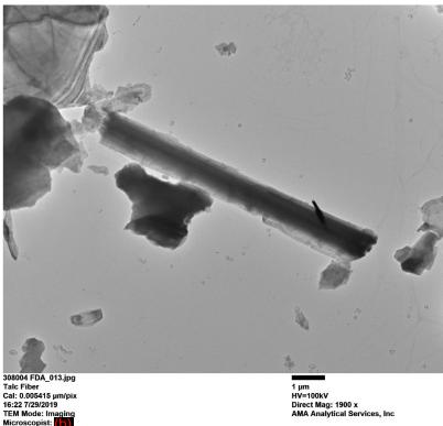
308004 FDA\_013.jpg Talc Fiber Cal: 0.005415 µm/pix 16:22 7/29/2019 TEM Mode: Imaging Microscopist: Imaging Microscopist: Camera: NANOSPRT5, Exposure: 800 (ms) x 5 drift frames, Gain: 1, Bin: 1 Gamma: 1.00, No Sharpening, Normal Contrast
