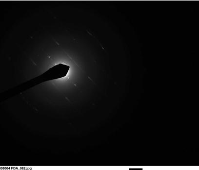
308004 FDA\_082.jpg Chrysotlie 2 15:45 87/2019 TEM Mode: Diffraction Microscopist: [11] Camera: NANOSPRT5, Exposure: 800 (ms) x 5 drift frames, Gain: 1, Bin: 1 Gamma: 1.00, No Sharpening, Normal Contrast
