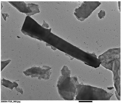
308004 FDA\_069.jpg Talc Fiber Cal: 0.003548 µm/pix 16:14 8/6/2019 TEM Mode: Imaging Microscopist: Camera: NANOSPRT5, Exposure: 800 (ms) x 5 drift frames, Gain: 1, Bin: 1 Gamma: 1.00, No Sharpening, Normal Contrast
