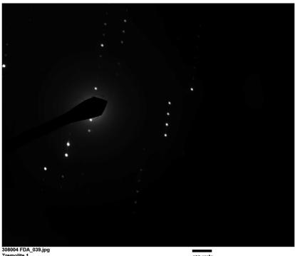
308004 FDA\_039.jpg Tremolite 1 17:57 7/29/2019 TEM Mode: Diffraction Microscopist [10] Camera: NANOSPRT5, Exposure: 800 (ms) x 5 drift frames, Gain: 1, Bin: 1 Gamma: 1.00, No Sharpening, Normal Contrast
