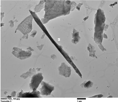
308004 FDA\_103.jpg Tremolite 3 Cal: 0.005415 µm/pix 15:55 8/8/2019 TEM Mode: Imaging Microscopist: Camera: NANOSPRT5, Exposure: 800 (ms) x 5 drift frames, Gain: 1, Bin: 1 Gamma: 1.00, No Sharpening, Normal Contrast
