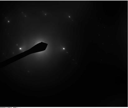
308004 FDA\_025.jpg Tremolite 3 17:08 7/29/2019 TEM Mode: Diffraction Microscopist: Camera: NAOSPRT5, Exposure: 800 (ms) x 5 drift frames, Gain: 1, Bin: 1 Gamma: 1.00, No Sharpening, Normal Contrast
