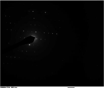
308004 FDA\_093.jpg Tremolite 1 14:45 8/8/2019 TEM Mode: Diffraction Microscopist: ()) Camera: NANOSPRT5, Exposure: 800 (ms) x 5 drift frames, Gain: 1, Bin: 1 Gamma: 1.00, No Sharpening, Normal Contrast
