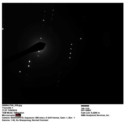
Zone-Axis Diffraction Pattern from the Tremolite Particle pictured above
