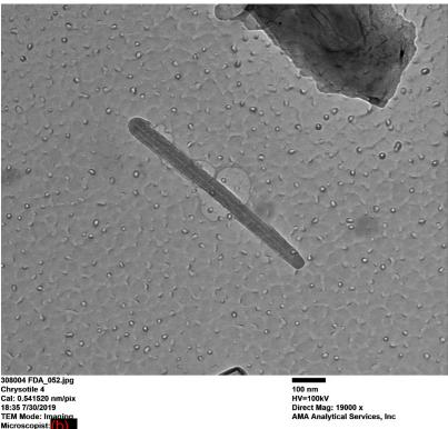
308004 FDA\_052.jpg Chrysotile 4 Cal: 0.541520 nm/pix 18:33 7/30/2019 TEM Mode: Imaging Microscopist: Anno Camera: NANOSPRT5, Exposure: 800 (ms) x 5 drift frames, Gain: 1, Bin: 1 Gamma: 1.00, No Sharpening, Normal Contrast
