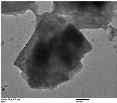
308004 FDA\_005.jpg Talc Cal: 0.001429 µm/pix 15:32 7/32/2019 TEM Mode: Imaging Microscopist. Camera: NANOSPRT5, Exposure: 800 (ms) x 5 drift frames, Gain: 1, Bin: 1 Gamma: 1.00, No Sharpening, Normal Contrast
