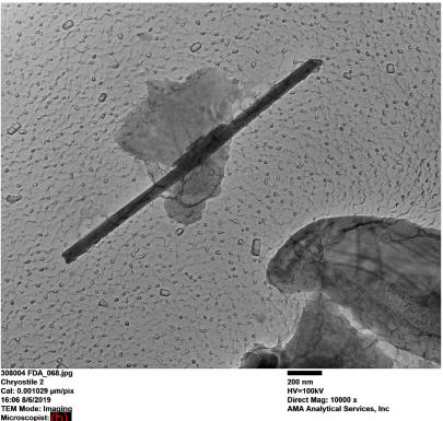
308004 FDA\_068.jpg Chryostile 2 Cal: 0.001029 µm/pix 16:06 8/6/2019 TEM Mode: Imaging Microscopist: Camera: NANOSPRT5, Exposure: 800 (ms) x 5 drift frames, Gain: 1, Bin: 1 Gamma: 1.00, No Sharpening, Normal Contrast
