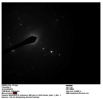
Diffraction Pattern from Tremolite Particle pictured above
