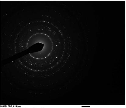
308004 FDA\_016.jpg Titanium particle or titanium coated particle 16:26 7/29/2019 TEM Mode: Diffraction Microscopist: (10) Camera: NANOSPR15, Exposure: 800 (ms) x 5 drift frames, Gain: 1, Bin: 1 Gamma: 1.00, No Sharpening, Normal Contrast
