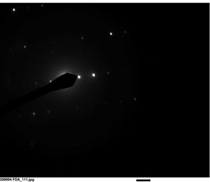
308004 FDA\_111.jpg Tremolite 4 17:06 8/8/2019 TEM Mode: Diffraction Microscopist. Camera: NANOSPRT5, Exposure: 800 (ms) x 5 drift frames, Gain: 1, Bin: 1 Gamma: 1.00, No Sharpening, Normal Contrast
