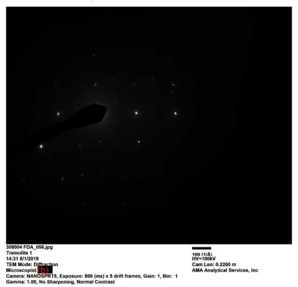
Diffraction Pattern from the Tremolite Particle pictured above
