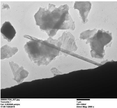
308004 FDA\_037.jpg Tremolite 1 Cal: 0.003548 µm/pix 17:55 7/29/2019 TEM Mode: Imaging Microscopist: Camera: NANOSPRT5, Exposure: 800 (ms) x 5 drift frames, Gain: 1, Bin: 1 Gamma: 1.00, No Sharpening, Normal Contrast
