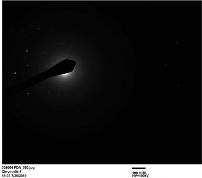
TEM Mode Diffraction TEM Mode Diffraction Microscopist: []] Camera: NANOSPRT5, Exposure: 800 (ms) x 5 drift frames, Gain: 1, Bin: 1 Gamma: 1.00, No Sharpening, Normal Contrast
