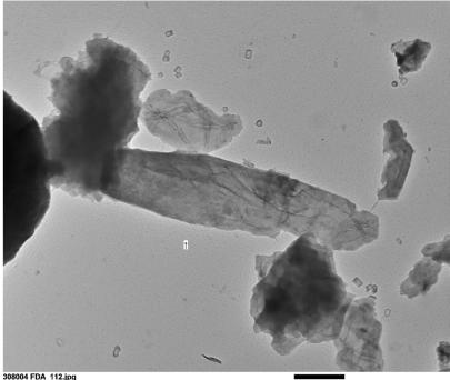
308004 FDA\_112.jpg Elongated Mica Particle Cal: 0.002858 µm/pix 13:12 8/12/2019 TEM Mode: Imaging Microscopist: (10) Camera: NANOSPRT5, Exposure: 800 (ms) x 5 drift frames, Gain: 1, Bin: 1 Gamma: 1.00, No Sharpening, Normal Contrast
