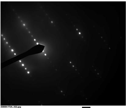
308004 FDA\_022.jpg Tremolite 2 16:51 7/29/2019 TEM Mode: Diffraction Microscopist [0] Camera: NANOSPRT5, Exposure: 800 (ms) x 5 drift frames, Gain: 1, Bin: 1 Gamma: 1.00, No Sharpening, Normal Contrast
