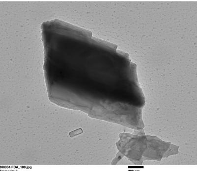
308004 FDA\_100.jpg Tremolite 2 Cal: 0.001029 µm/pix 15:33 8/8/2019 TEM Mode: Imaging Microscopist: Camera: NANOSPRT5, Exposure: 800 (ms) x 5 drift frames, Gain: 1, Bin: 1 Gamma: 1.00, No Sharpening, Normal Contrast
