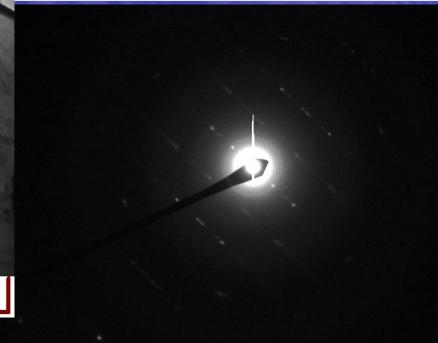
1200EX 7/3/2012 HT: 100 kV Exposure Time: 10.00 Sec Camera Length: 80cm NYT-3a: Chrysotile
