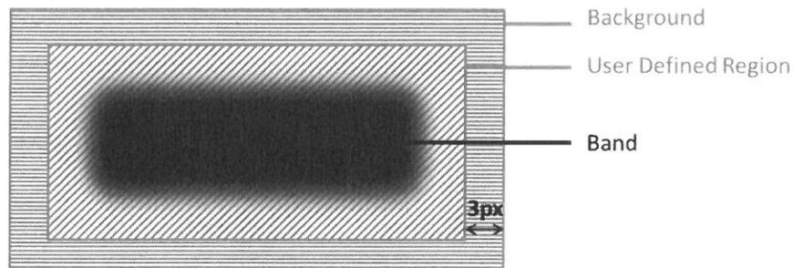
**Figure 1a:** Schematic representation of a 'UDR' (diagonal stripes), the 'Background' which is a perimeter 3 pixels wide surrounding the 'UDR' (horizontal stripes) and a 'Band' within the 'UDR'. 3px abbreviation denotes the three pixel perimeter.
