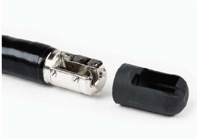
During reprocessing, removal of the distal cap allows greater access to the elevator, including the underside of the elevator. This type of design is predicted to improve the ability to clean the elevator recess, and thus improve the safety of these devices.
