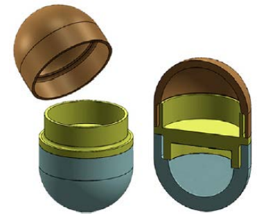
3D printed multicompartmental capsule
