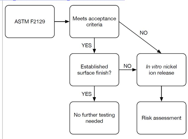
Figure 1. Corrosion testing paradigm flowchart
