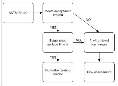
Figure 1. Corrosion testing paradigm flowchart
