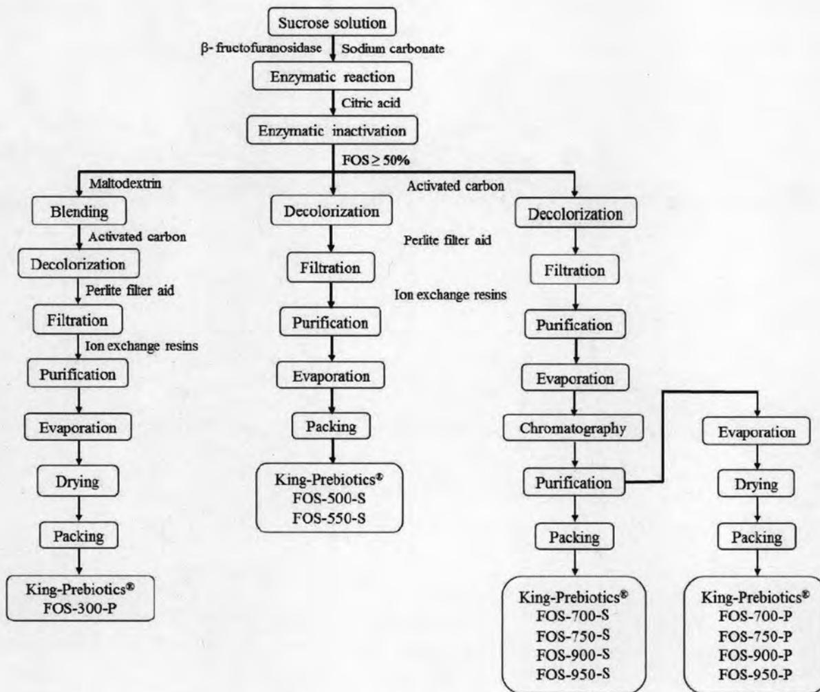
Figure II.G.1. Manufacturing Process of FOS
