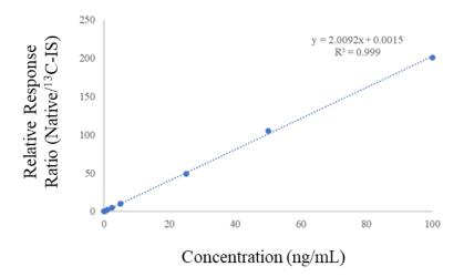
Step 2: Calculate mycotoxin concentration in test sample.
