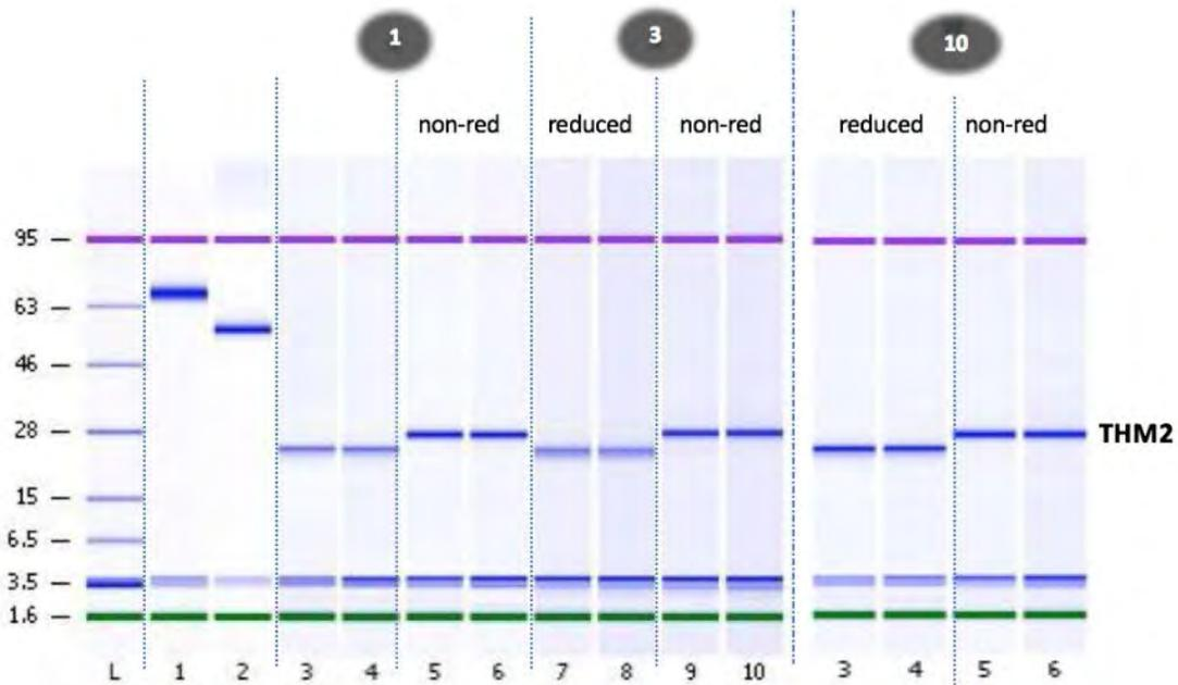
**Figure C-3. Purity of heat-extracted thaumatin II by CGE**
