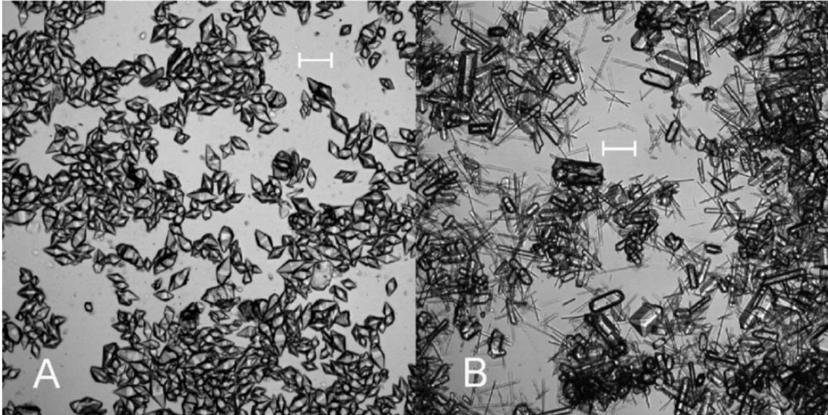
**Figure C-8. Crystals of thaumatin obtained by precipitation with tartrate**
