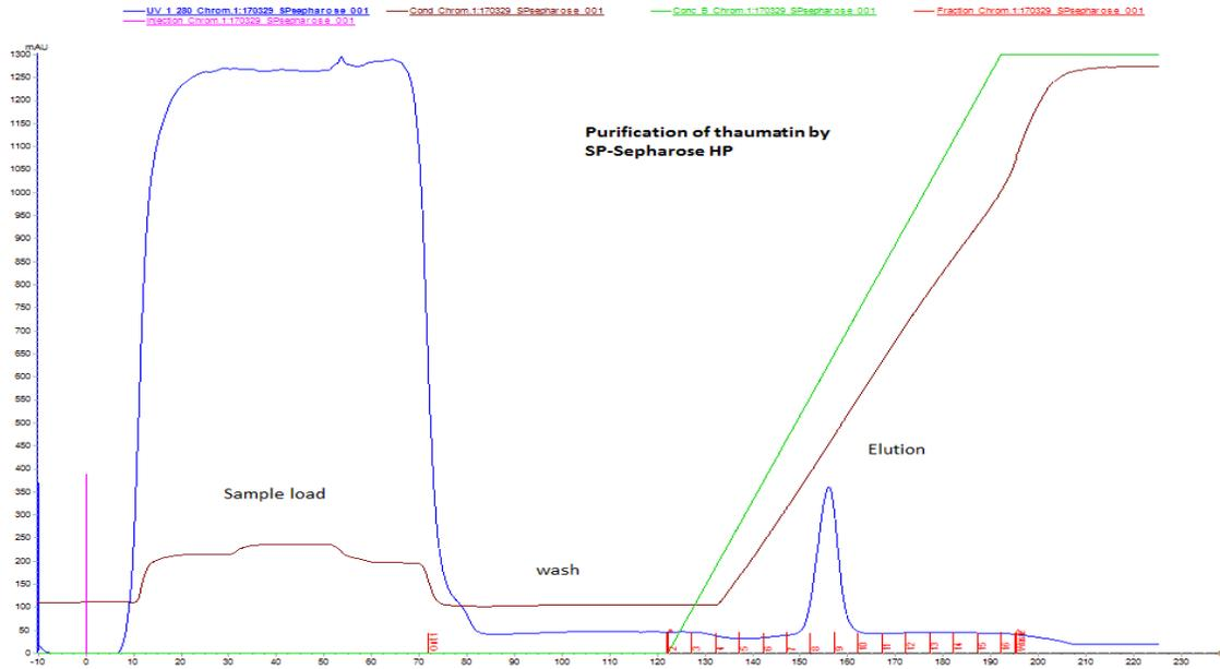
**Figure C-6. One-step purification of cold-extracted thaumatin by SP Sepharose HP chromatography**
