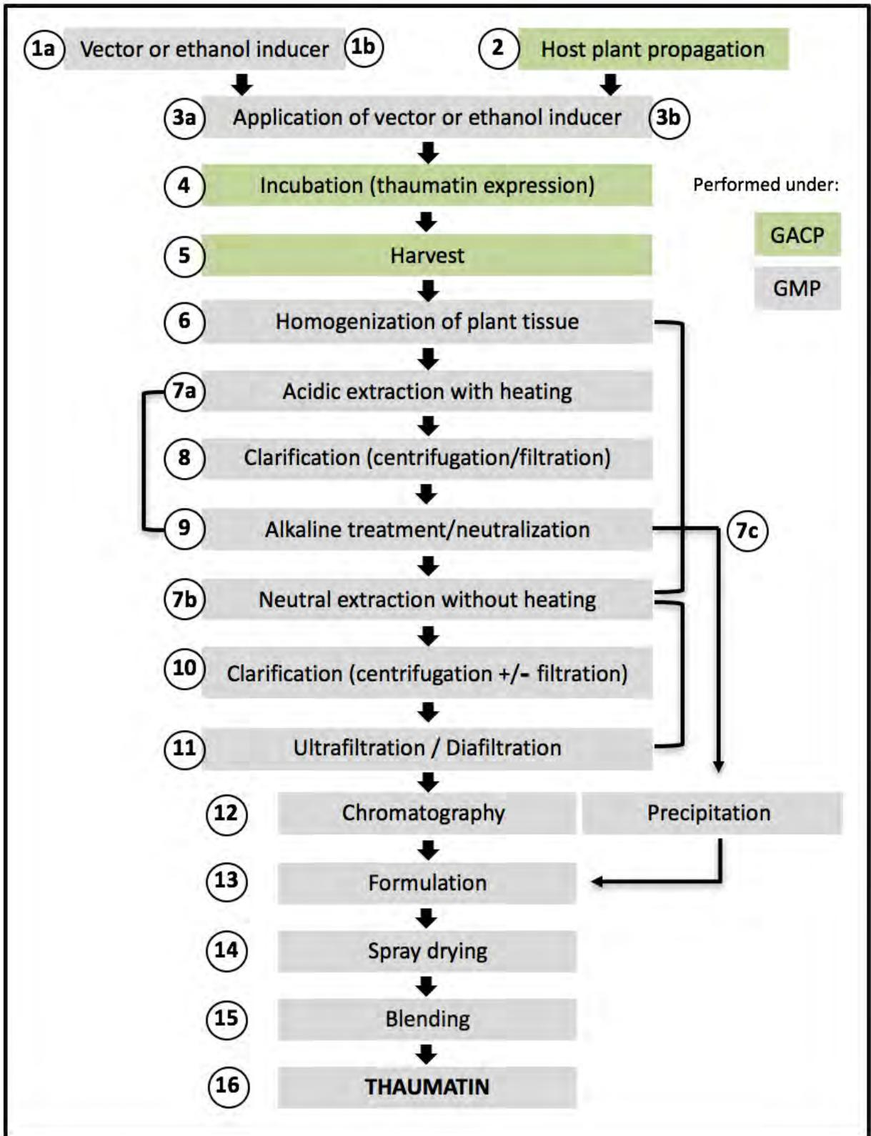
Figure B-3. Summarized process diagram for THAUMATIN production in plants
