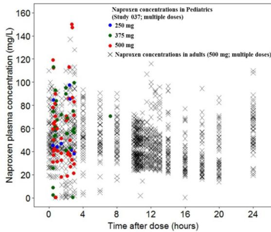
Figure 3. Naproxen concentrations from Study 037 compared with the mean naproxen PK profile in pediatric patients who took the approved dose of naproxen for Juvenile Arthritis (5 mg/kg as naproxen suspension)
