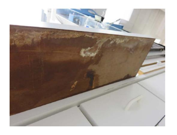
View of the bottom surface of the ISO 5 LAFW showing wood like surface that appears to be stained.
